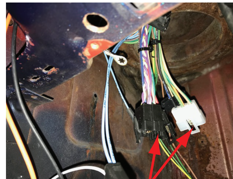
5. Your engine (510466) and front light (510465) harnesses will plug onto these 4 dash leads, will route out to the Engine Compartment. The final connection details are shown on pages 16,17, 18 and 19 of this instruction set.
