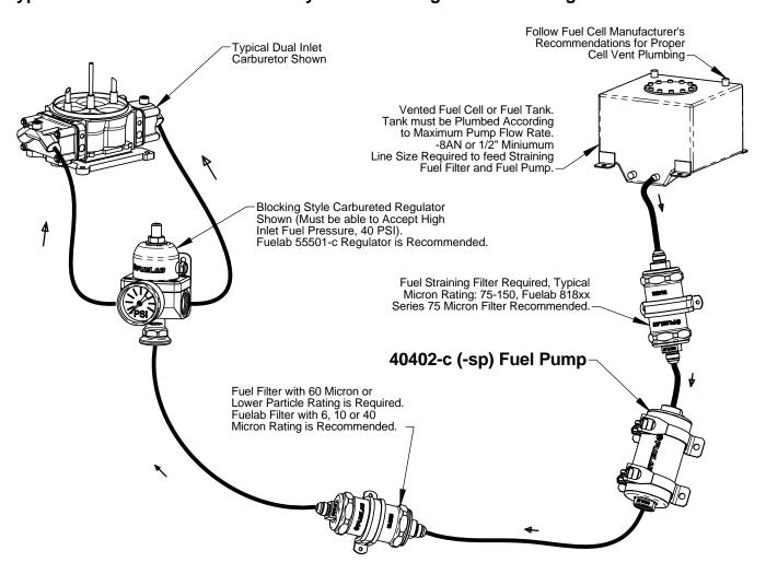
Special Note: Fuel Pump can be used with a bypass return or relief valve style regulator as well. For extended periods of operation, Fuel Pump must operate in reduced speed mode ONLY.
