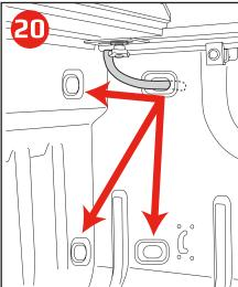
Route the front drain hoses from the end of the BAKFlip rail out through manufacturer available bed plug. Simply remove these plugs or drill a 7/8" hole through the plastic. If you have a drop in plastic bedliner, simply run the drain tubes behind or under the liner.
