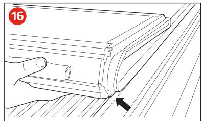
Unfold the cover towards the tailgate. Make sure the cover fits squarely between the rails.
