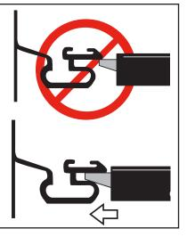
Sometimes, your side seals of your BakFlip cover will appear to be wrinkled shortly after initially installing the cover. To assist seals in laying flat you can leave your truck in the sun, or to expedite, just apply heat with a hair dryer or heat gun. See this video for a good look at how it's done.
