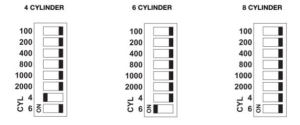
8. Select the rev limit using the 6 top switches. The minimum rpm (with all switches in the "off" position) is 5,000 rpm. For higher rpm limits, add the value of the switches in the "on" position to the base setting of 5,000. See the examples below.
