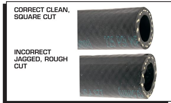
Figure 5 Severing the Hose Properly.
