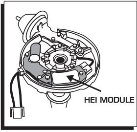
Figure 1 Replacing the Module.
