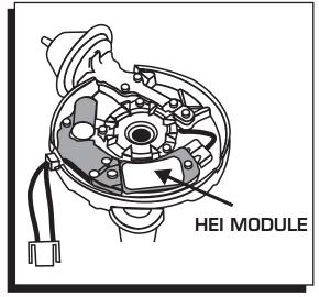
Figure 1 Replacing the Module.
