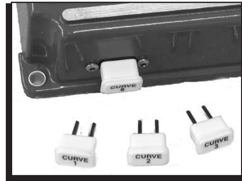
Figure 3 Timing Curve Modules.
