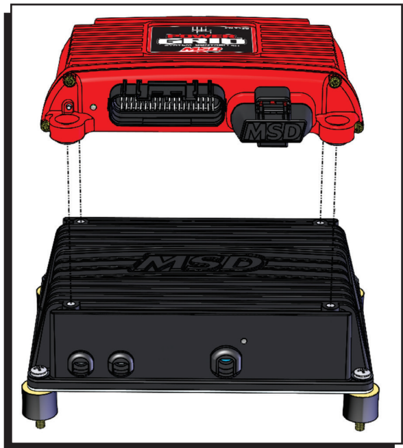
Figure 4. Power Grid Mounted Install
