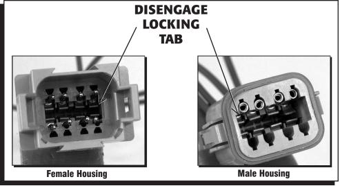
To remove the terminals and wires, use a small screwdriver or awl to disengage the locking tabs and pull the wire out (Figure 9).
