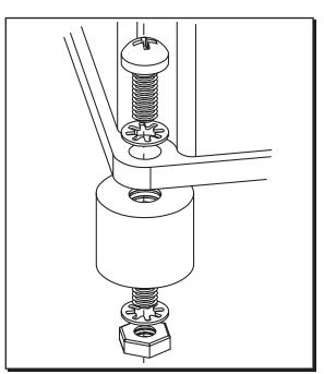
Figure 1 Mounting the Points Box.
