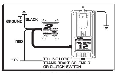
Figure 6 Wiring a Two Step.
