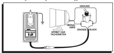
Figure 5 Wiring a Two Step.
