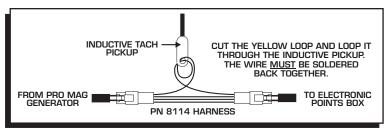
Figure 4 Wiring an Inductive Triggered Tach.
