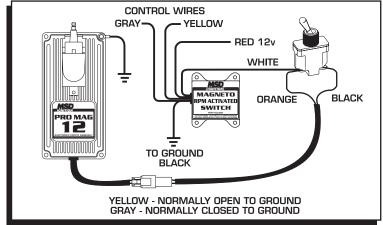
Figure 7 Wiring an RPM Activated Switch.
