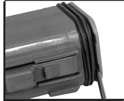
Figure 5 Disassembling the Male Housing.
