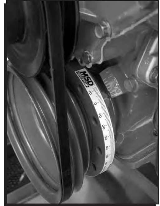
Figure 9 The Timing Tape Installed.
