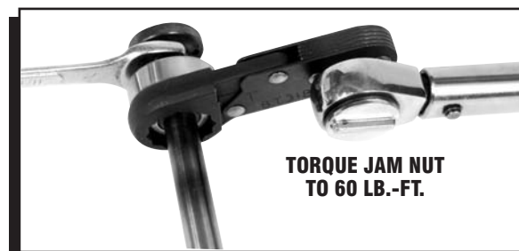
Figure 11 Installing the New Bearing and Lock Nut.
