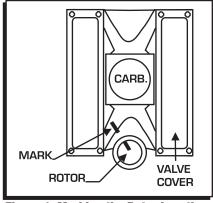
Figure 1 Marking the Rotor Location.
