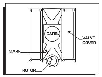
Figure 8 Marking the Rotor Location.
