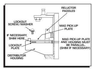
Figure 13 Checking Installation of the Lockout Plate.
