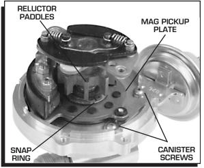
Figure 12 Removing the Vacuum Canister.
