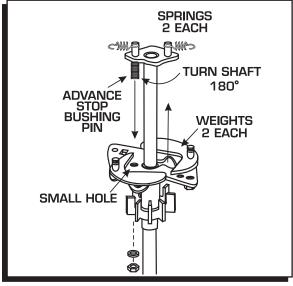
Figure 7 Locking Out the Advance.
