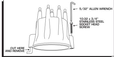
Figure 14 Optional Installation by Bolting the Cap Down.
