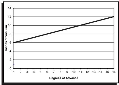
Figure 11 Vacuum Advance and Timing Chart.
