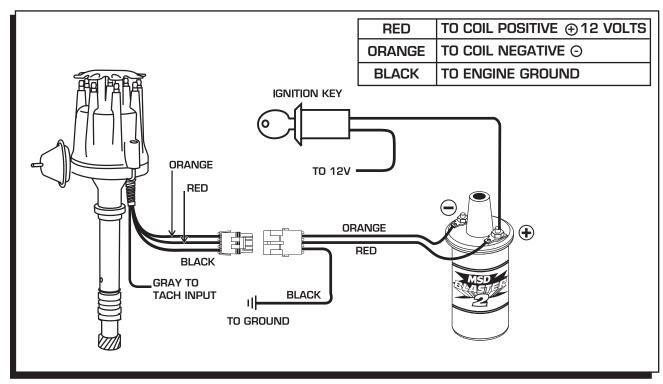
Figure 9 Wiring the Ready-to-Run Chevrolet Distributor.
