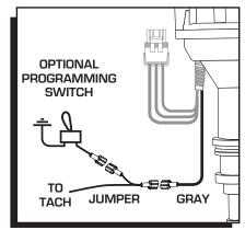
Figure 15 Setting the Rev Limiter.
