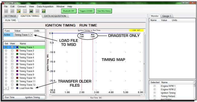
Figure 3 View Software Ignition Timing Screen.
