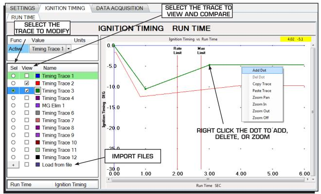
Figure 4 View Software Ignition Timing Screen.
