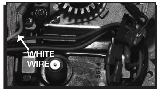
Figure 8 Routing the MSD Wiring.
