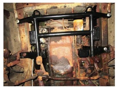
14. Re-check all fasteners to ensure they are tight and new cotter pins have been placed into the lower ball joints.
