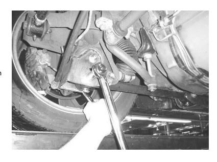
Note: It is highly recommended that you run QA1 boxed control arms P/N 5204. Stock arms tend to flex and twist under hard acceleration and aggressive cornering.
