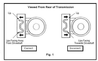
driveline misalignment and possible damage to the transmission, drive shaft, u-joints, rear axle, torque arm, and/or floor pan of vehicle. We highly recommend using a good polyurethane transmission mount. This will ensure your transmission will stay solid and the torque arm will work to its full potential.
