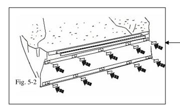
(b) Attach 1" X 60" and 1" X 2" hook to the BedRug bulkhead area facing the front as shown. Trim excess from 1" X 60" strip where necessary. **Do not remove adhesive protective film at this time**. (Fig. 5-2)
