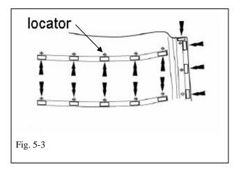
(b) Attach 1" X 2" fasteners to the back sides of the BedRug sidewalls as marked by locators. **Do not remove adhesive protective film at this time.** (Fig 5-3)
