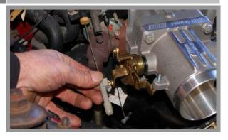
Re-install the throttle cables and return spring.
