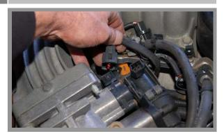
Unplug the TPS and IAC valve electrical connections.
