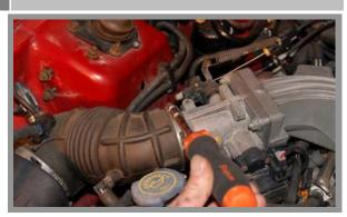
Remove the Air Temperature Sensor from the inlet tube. Loosen the clamps on the inlet tube at the throttle body and at the air box.
