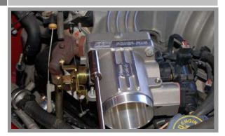
Install the provided gasket and throttle body onto the intake using the stock nuts and tighten.
