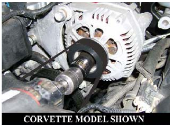
Pic. 1 Loosen alternator nut
