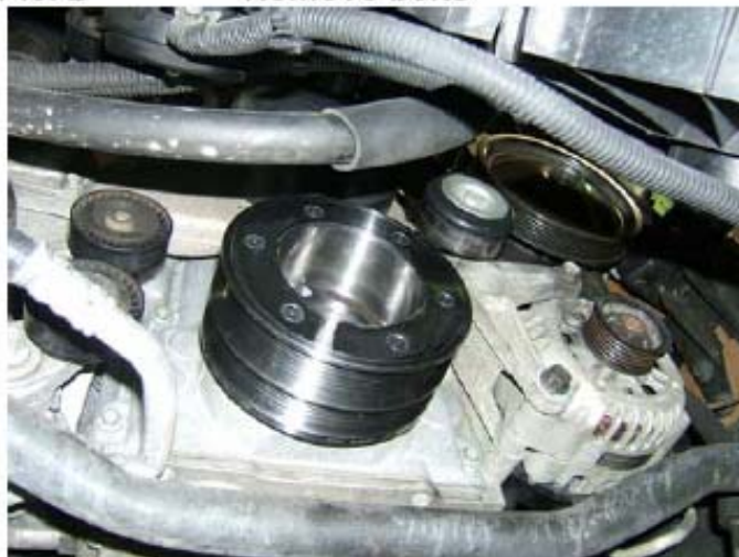
Pic. 4 Crank pulley/balancer installed
