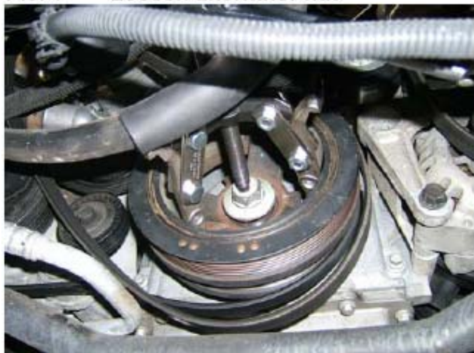
Pic. 3 Using the puller tool
