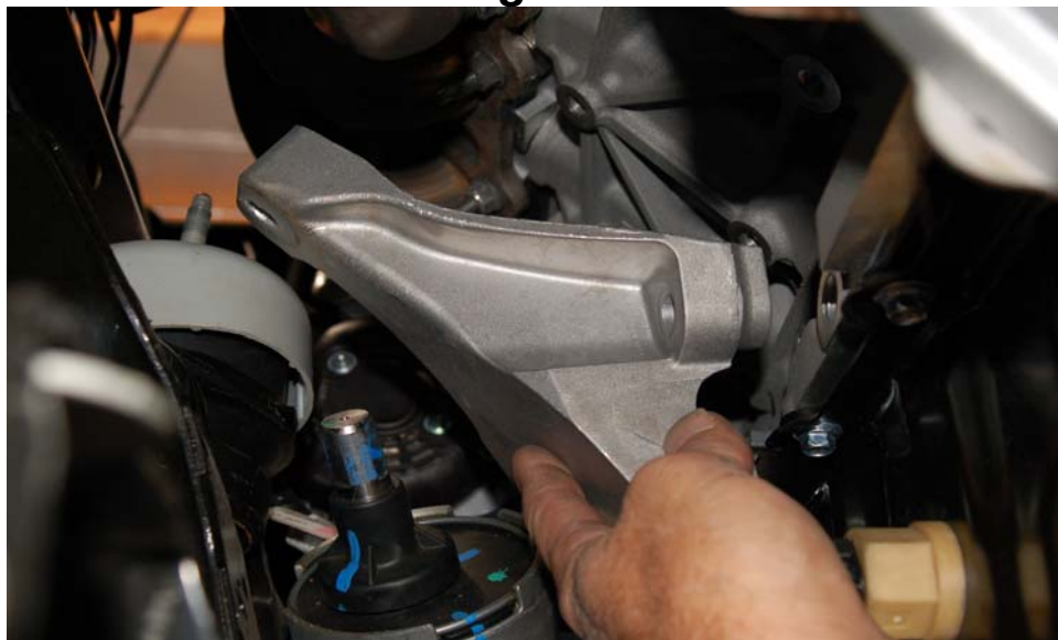
Motor mount removal.
