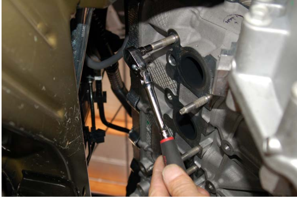
Removing stock studs.
