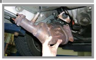
Remove the nuts that connect the catalytic converters to the exhaust manifolds, and then remove the converters from the vehicle.
