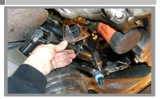
Remove the bolts that attach the steering shaft to the steering rack and firewall steering column yoke.
