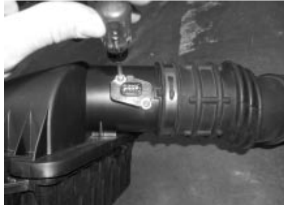
Remove mass air meter.
