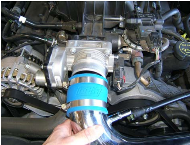
Make connection at throttle body.
