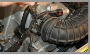
• Unplug the air temperature sensor on the stock inlet tube. Remove the sensor for re-use in the BBK inlet tube. Loosen the clamp at the throttle body.
