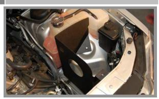
Place the filter shield into place in the engine compartment and line up the grommet with its hole. Mount the front tab of the filter shield using the stock bolt.
