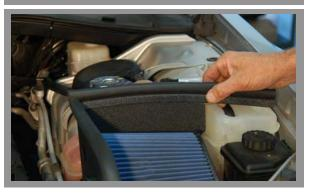
From the supplied hardware kit, find the aluminum pin and 1/4" Phillips screw and install on the BBK filter shield. Install the stock rubber grommet onto the pin. Install the supplied sponge rubber seal to the top of the filter shield. **STEP 6**
