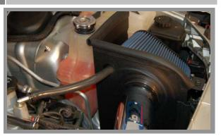
• Place the supplied filter into the shield area and push the neck of the filter base, where the clamp mounts, through the opening in the filter shield. Install the BBK Inlet Tube into the filter and into the blue hose connector. Position for the best fitment and be sure the opening in the base of the filter lines up with the smaller hole in the filter shield. Then tighten the clamps.
