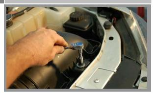
Remove the bolt that mounts the front of the air box to the vehicle. Lift out the air box and remove with the inlet hose.
