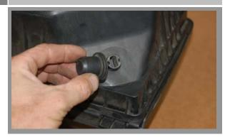
• On the bottom rear of the stock air box, remove the rubber grommet for re-use with the BBK filter shield.
