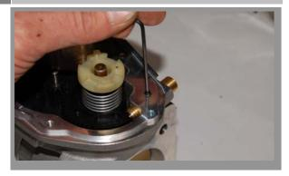
With a 2.5mm allen wrench, loosen the set screw for the brass adjuster stud.
