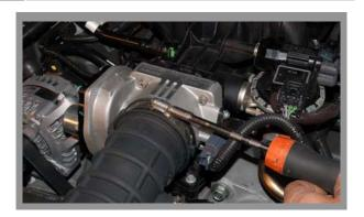
Re-install the air intake tube and connect the breather tube. Reconnect the negative battery terminal.
