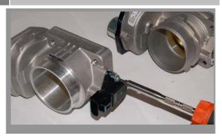
• Remove the TPS sensor and re-install on the BBK Throttle Body using the stock screws.
