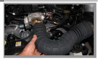
Disconnect the breather tube from the air intake tube. Loosen the clamps at the throttle body and at the air box then remove the air intake tube.
