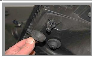
• Remove the bolt on the right side of the air box that mounts it to the inner fender. Detach the air box from the lower inlet tube on the side of the radiator as you remove the air box. Detach the Mass Air Meter wire harness from the side of the air box by slightly pulling on the harness on each barbed mounting pin. Also remove the 2 bottom rubber grommet for the air box.
