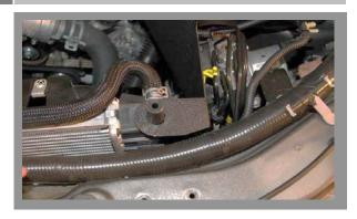
Install the BBK Air Filter Shield into place and position over the radiator mount peg with the rubber grommets seating into their holes in the inner fender. Install the stock bolt back into the small tab on the shield and tighten the bolt. Reinstall the upper radiator mount and tighten the bolts.
