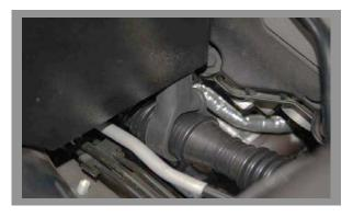
Route the sound tube under the plastic breather hose, so sound tube will pass under BBK cold air shield. Use the stock rubber clamp to retain the sound tube to the bottom of the filter shield.
