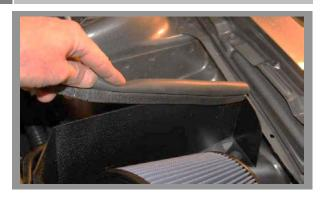
Install the supplied spongy trim to the top of the Air Filter Shield and cut off any excess trim.
