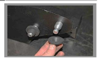
Assemble the 2 aluminum pins to the bottom of the BBK Air Filter Shield using the supplied ¼-20x1/2" Phillips screws. Install the stock rubber grommets onto the pins.
