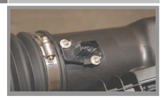
Remove the Mass Air Sensor from the stock air box tube. Install in the aluminum mounting base on the BBK inlet tube with the 2 supplied 4mm
