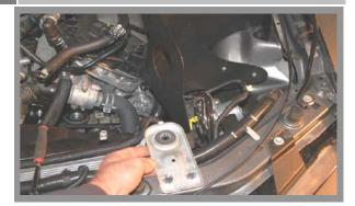
Remove the 2 bolts that retain the driver side radiator mount and remove the mount.
