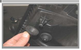
Remove the bolt on the right side of the stock air box that mounts it to the inner fender. Detach the air box from the lower inlet tube on the side of the radiator as you lift the box out to remove. Detach the Mass Air Sensor wire harness from the side of the air box by slightly pulling on the harness at each barbed mounting pin. Remove the 2 rubber grommets from the bottom of the air box.
