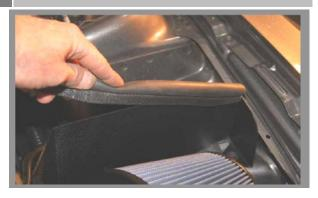
Install the supplied sponge seal to the top of the air filter shield and trim off any excess
