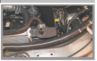
Install the BBK air filter shield into place and position over the radiator mount peg with the rubber grommets seating into their holes in the inner fender. Install the stock bolt back into the small tab on the shield and tighten the bolt. Reinstall the upper radiator mount and tighten the bolts.
