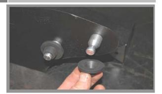
Assemble the 2 aluminum pins to the bottom of the BBK air filter shield using the supplied 1/4-20x 1/2" Philips screws. Install the stock rubber grommets onto the pins.
