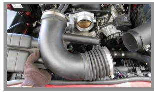
Disconnect plastic breather hose from tube at the passenger side valve cover. Now remove the Air Inlet Tube from the vehicle.
