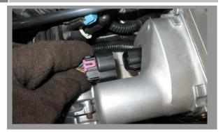
Disconnect the electrical connector at the throttle body. Remove the four 10mm bolts that secure the throttle body to the intake manifold and place it on a workbench. NOTE!!! Be careful when disconnecting. Because of some TSB's from GM about the connector wires becoming loose easily, be sure to pull from the connector and NOT from the wires when disconnecting from the throttle body.
