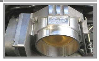
Install the BBK Throttle Body using the supplied hardware (The Factory O-Ring is re-used), plug in the electronics, re-install the Air Inlet Tube and breather hose. Tighten the hose clamps. NOTE!!! If installing the 102mm BBK Throttle Body you will have to install the provided spacer between the manifold and throttle body. Also be sure that the supplied O-ring is installed in the machined groove on the spacer, and the factory o-ring is clean and not damaged.
