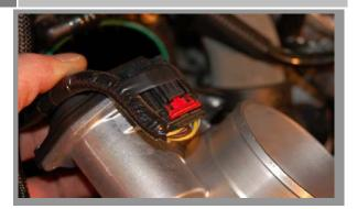
Remove the four mounting bolts from the stock throttle body, as you remove the throttle body, flip it to unplug the motor plug on the bottom.
