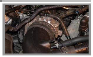
Re-install the air inlet tube and reconnect the breather tube. A little WD-40 or light grease on the inside of the tube may help in this process. Tighten the clamps.
