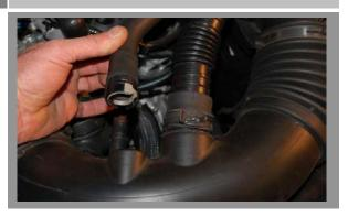
Disconnect the smaller plastic breather tube from the air inlet tube. You can leave the sound tube connected.
