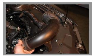
Remove the air inlet tube and set it aside.
