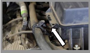
Loosen the two 10mm mounting bolts that secure the factory intake system to the vehicle. Also remove the clip on the passenger side of the stock intake system using pliers.
