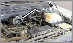
Unclip the three clips at the air box and remove the entire system out of the vehicle. NOTE!!! The rubber coupler also needs to be removed from the throttle body.
