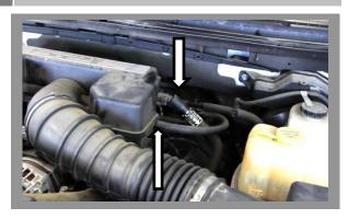
Remove the two vent hoses going into the factory intake system.
