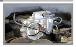
Disconnect the electrical connector at the throttle body and remove the throttle body from the vehicle.
