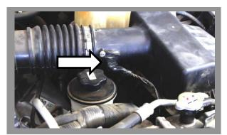
Disconnect the Mass Air Flow (MAF) Sensor.
