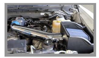
Install the supplied Air Filter, plug in the MAF Sensor and be sure all the clamps are tight.
