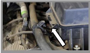
Loosen the two 10mm mounting bolts that secure the factory intake system to the vehicle.
