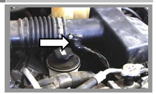
Disconnect the Mass Air Flow (MAF) Sensor.
