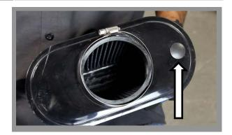
Install the sponge trimming onto the BBK Cold Air Intake shield and install the supplied plug into the BBK Air Filter.
