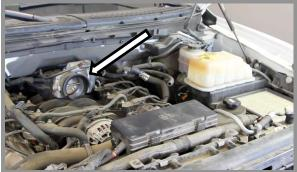
Unclip the three clips at the air box and remove the entire system out of the vehicle.
