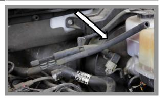
Remove the factory vent hose and replace it with the supplied 3/8" hose. Connect the supplied 3/8" hose to the plastic straight fitting on the BBK Intake Tube. The Valve Cover vent hose with the clip will be connected to the larger welded tube coming off the BBK Intake Tube. NOTE!!! Be sure that the clipped vent hose is pushed onto the welded tube until it clicks into place.
