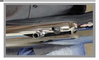
Install the supplied rubber grommet and straight fitting into the BBK Cold Air Tube.
