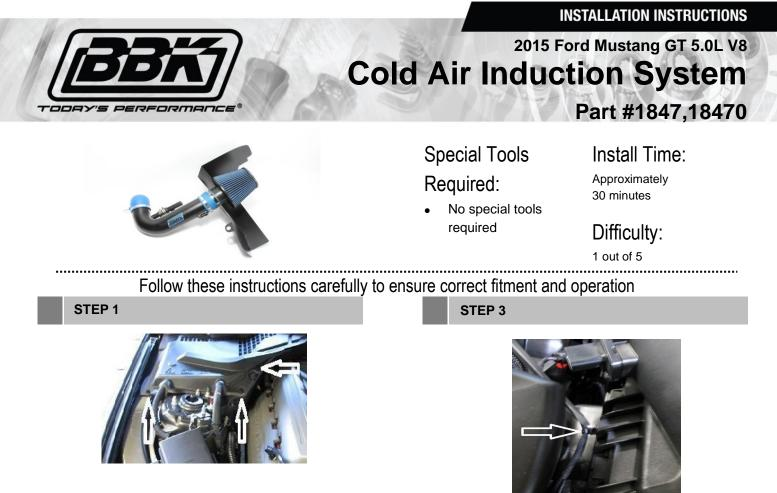
Remove the 3 screw pins that hold the battery cover to the body lift up the battery cover and disconnect the negative battery terminal. Remove the engine cover by pulling it upward releasing it from its rubber grommets.
