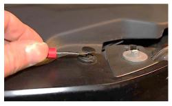
• Remove the plastic radiator cover by prying up the center of the plastic pin heads at the slots cut on each side pull all the pins out and set the cover to the side.
