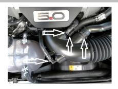
Disconnect the 3 breather hoses and the sound hose from the inlet tube. Loosen the clamps on the inlet tube at the throttle body and the air box, remove the inlet tube from the vehicle.
