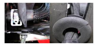
• Pull back the spongy trim on the air shield. Take the rubber grommet supplied in the kit and cut a slit into it so that it can be opened up and slid over the wiring harness for the mass air flow sensor. Once it is placed on the wiring harness slide the grommet and wiring harness down the cut out on the air shield until it is in place, push the spongy trim back onto the air shield.
