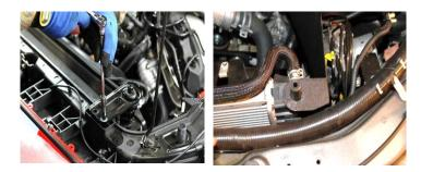
Remove the 2 10mm bolts from the driver side radiator mount and remove the mount by pulling it upwards from the vehicle. Install the BBK Air Filter Shield into place by setting it straight down onto the radiator mount peg. Install the stock bolt thru the air shield and bolt it back into the small tab on the inner fender. Reinstall the upper radiator mount and tighten the 2 bolts.
