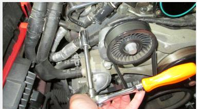
Using 15mm socket and extension remove factory engine harness nut leaving harness in place.
