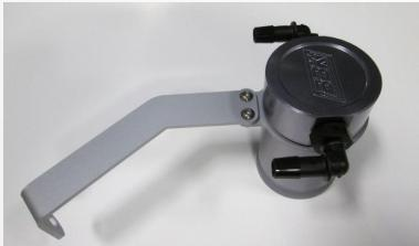
Assemble oil separator by installing o-ring bracket onto separator by removing cap. Now screw cap back down aiming towards top of BBK logo also install supplied fittings using 17mm wrench in the same direction. Now install bracket and allen bolts using a 3/32 allen wrench as show in photo.
