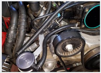
Now install new BBK oil separator assembly as shown in picture and tighten nut. When running hoses to oil separator run your first hose from the plastic fitting on intake manifold to the filtered side of oil separator as shown in picture. Then run the other hose from steel tube below intake manifold to the other side of the oil separator. This is the pressure side.
