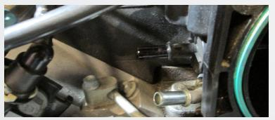
Remove factory air box and throttle body to help in removal of factory crossover hose and install of BBK oil separator kit. Remove factory hose by pushing aside the factory clip and pull outwards.
