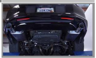
With all the clamps snug, make any fitment adjustments starting at the front clamps on the mid pipe and ending at the muffler tips, then tighten.
