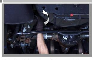
Twist the mid pipe so the muffler has enough clearance to be removed.
