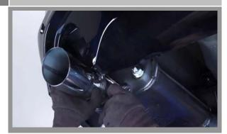
Slide and snug the exhaust tip onto the outlet tube of the muffler.
