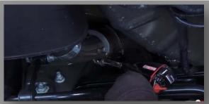
Starting on the driver side, loosen the clamps at the mufflers and mid pipes.
