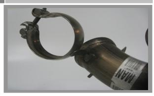
NOTE!! On 2011-2013 Models you will need to remove the factory clamp from the stock muffler to use on the inlet tube for the BBK Axle Back System. The clamp has a very small and brittle tack weld on it only for the factory production line use. Its easily removed by cutting or wiggling the clamp back and forth until it breaks off the stock muffler.
