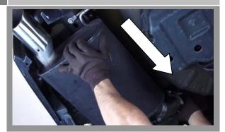
Slide the muffler towards the front of the vehicle and remove.
