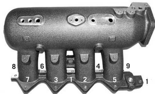
Diagram B TORQUE SEQUENCE
