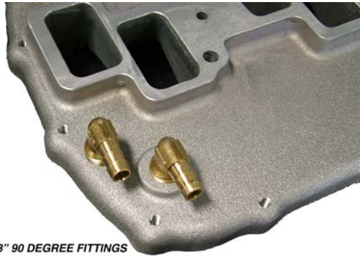
3/8" 90 DEGREE FITTINGS POINTING OUT TO DRIVER SIDE FOR CONNECTION TO BRAKE BOOSTER & VACUUM TREE.
