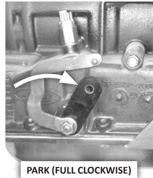
19. Move the selector lever to PARK (fully clockwise), then move it to OD (3 clicks back).
