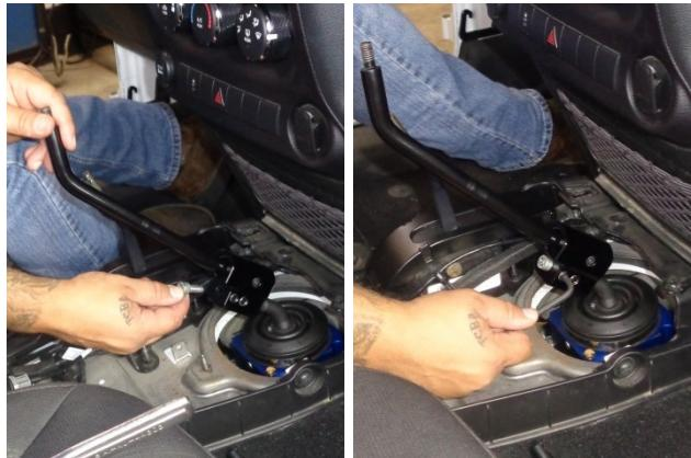
6. Press the shift stick and adapter (item 3) onto the vehicle's shift lever and secure with the original bolt, then tighten the two set screws on the side of the adapter.
