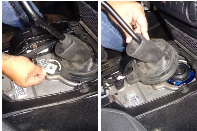
4. **CAUTION: The sheet metal nut plate has sharp edges!** Carefully remove the sheet metal nut plate, then remove the shifter boot.
