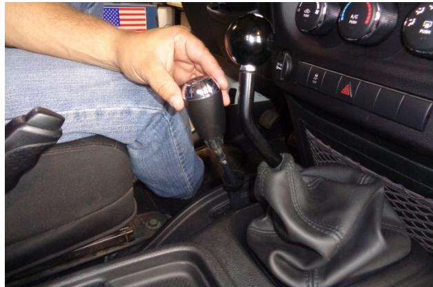
10. Reinstall the trim ring and shift knob on the transfer case shift lever, then snap the trim ring to the bottom of the knob to secure it to the lever.
