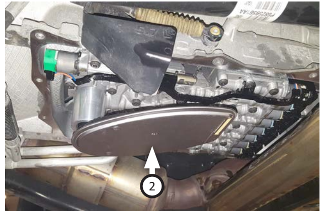
9. Install o-ring (5) onto filter extension (3) then attach it onto deep pan filter (2). Install filter assembly onto transmission oriented as shown.
