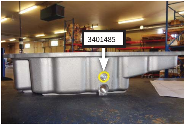
11. This kit includes a 1/8 NPT port above drain plug that can be used for an optional transmission temperature gauge. (available separately) Otherwise, install pipe plug (3401485) in port.
