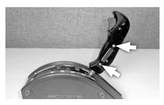
**15.** Tighten the pistol grip set screws in an alternating manner until they are flush with the grip. Test the trigger to verify that it actuates and resets smoothly.
