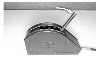
**13.** Move the shift lever to LOW (1), which will allow the lockout plunger on the pistol grip to align more easily with its guide hole inside the lever.
