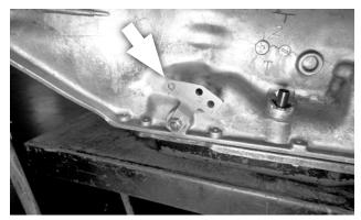
17. At the transmission, install the B&M selector lever using the stock selector lever nut, and tighten the nut to 23 ft-lbs torque. The lever should travel smoothly back and forth, with a positive "click" in each detent.
