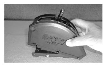
12. Ensure there is no debris in the shifter mechanism. Then reinstall the gate plate and cover assembly on the shifter base while guiding the shift lever up through the NEUTRAL position. Secure the cover to the shifter base with 3 screws on each side.
