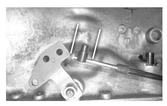
21. Thread the swivel onto the cable to about the middle of the threaded section, then install (but do not yet tighten) the jam nut.
