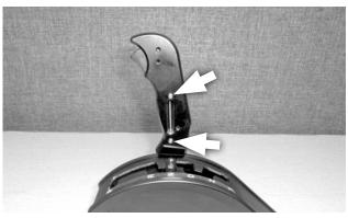
**3.** Loosen the 2 grip set screws 2-3 turns, then remove the pistol grip assembly from the shift lever.
