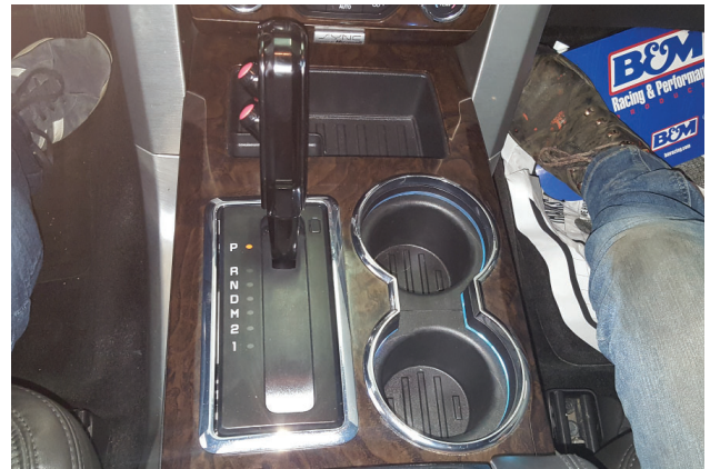
16. Tuck any wiring aside, making sure to avoid moving components, then put cupholder back into place as shown.
