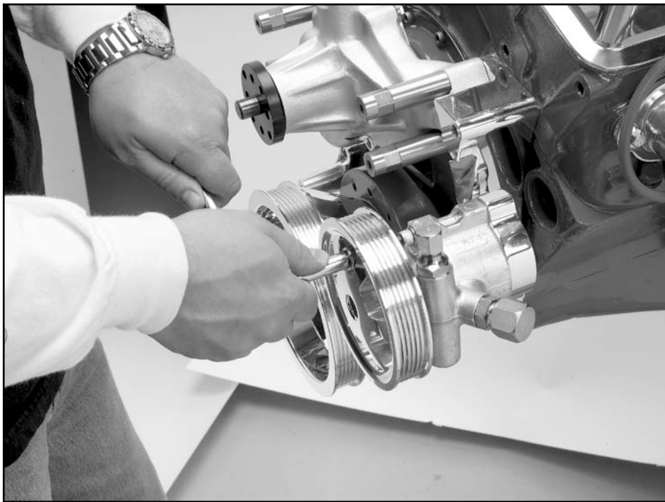
Figure 11: Install Power Steering Pump & Pulley
