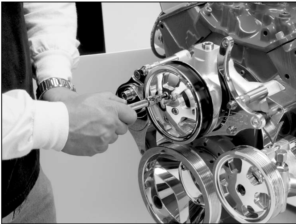
Figure 15: Install Water Pump Pulley
