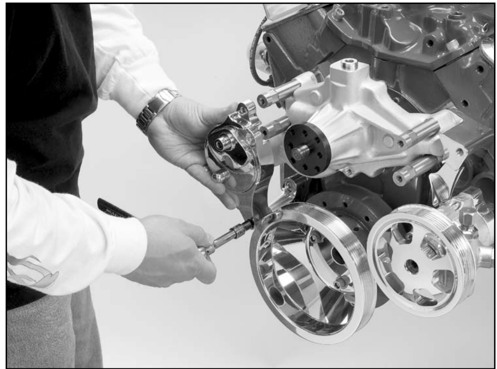
Figure 12: Install Belt Tensioner
