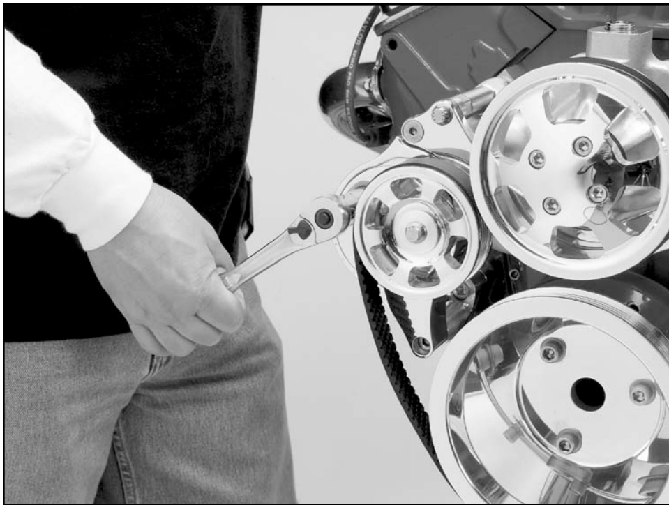
Figure 19: Install Serpentine Belt
