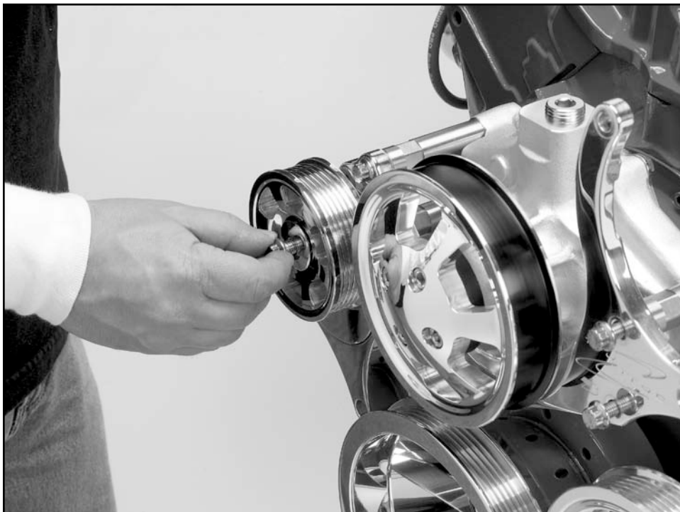
Figure 17: Install Tensioner Pulley
