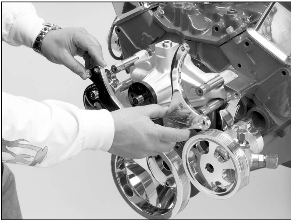
Figure 13: Install Bridge Bracket
