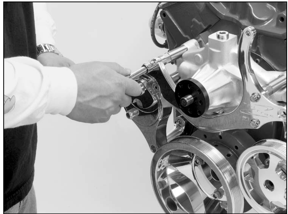
Figure 14: Bridge Bracket Tightening Instructions
