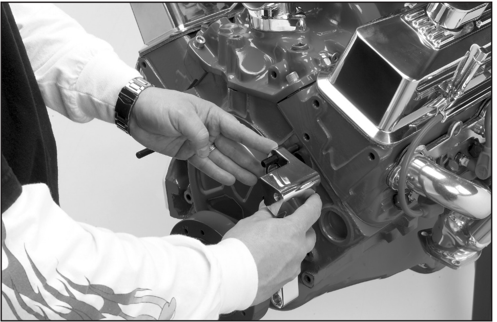
Figure 4: Install Alternator Bracket
