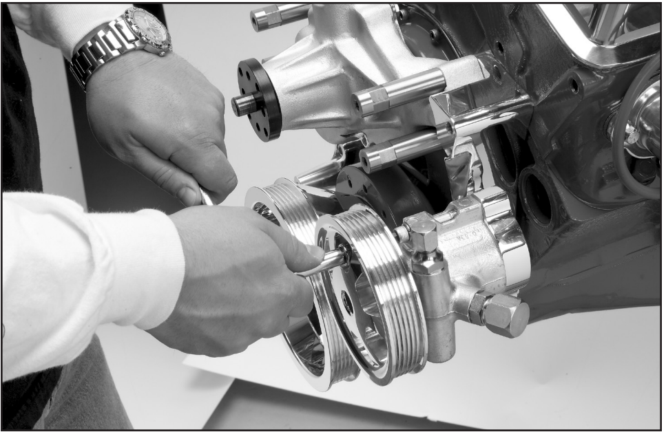
Figure 11: Install Power Steering Pump & Pulley
