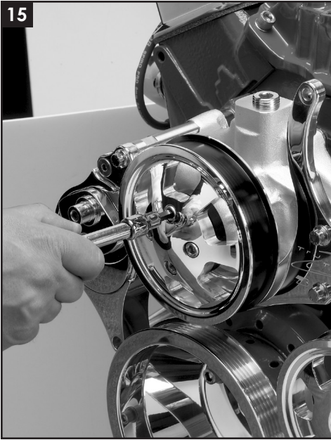
Figure 15: Install Water Pump Pulley
