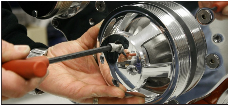
Figure 12: Install Water Pump Pulley
