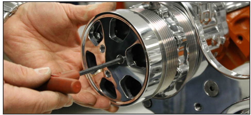
Figure 13: Install AC Clutch Cover
