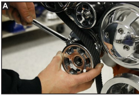
Figure 15: Install Belt & Tensioner Pulley
