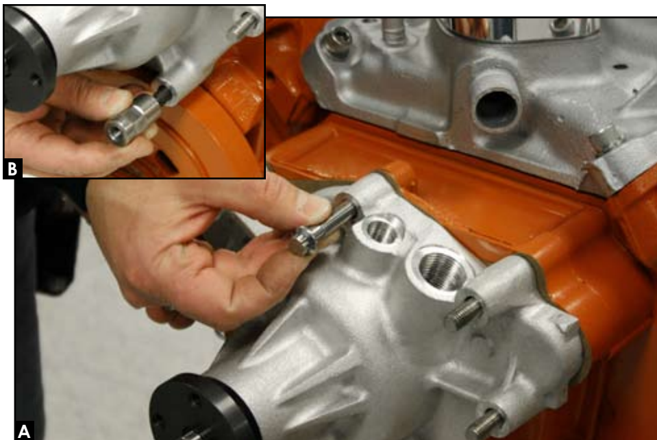
Figure 3: Install Water Pump
