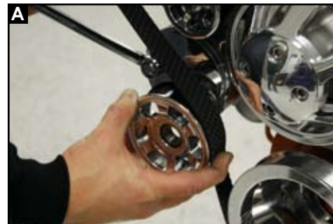
Figure 15: Install Belt & Tensioner Pulley
