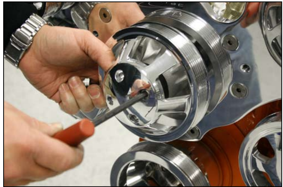
Figure 12: Install Water Pump Pulley
