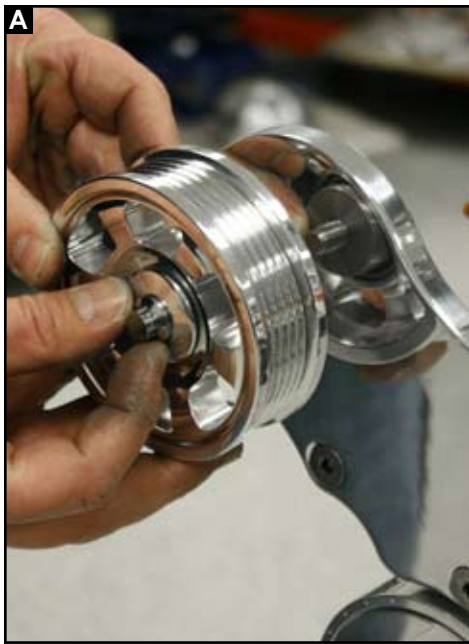
Figure 13: Install Idler Pulleys
