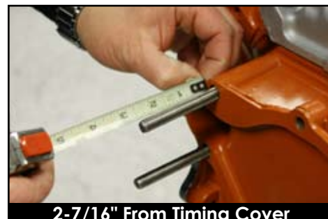
Figure 2: Install Block Mounting Studs
