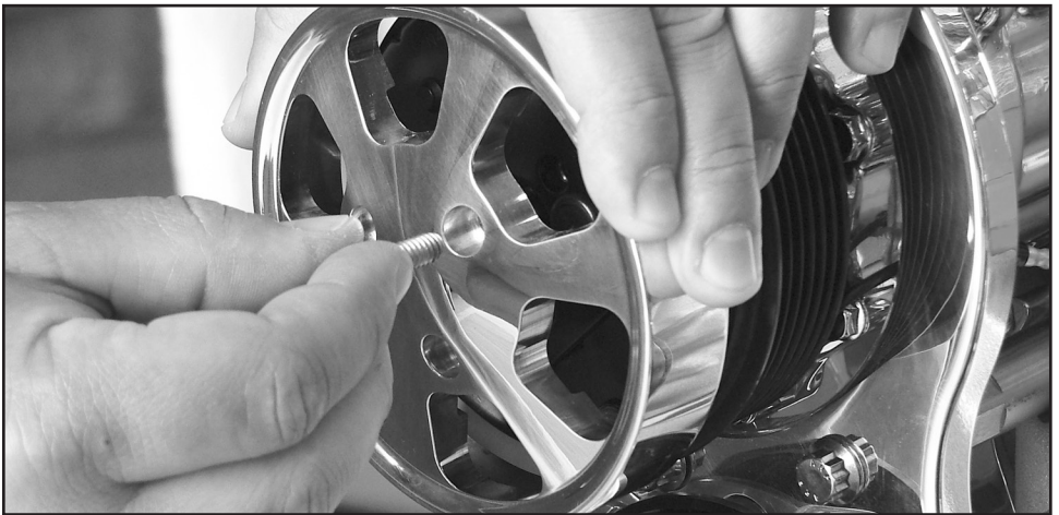
Figure 13: Install SD-7 Compressor Clutch Cover
